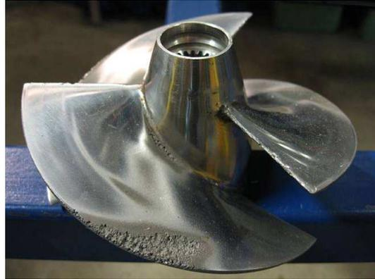
Figure 1.1: Cavitation damage on a propeller blade<sup>1</sup>.
