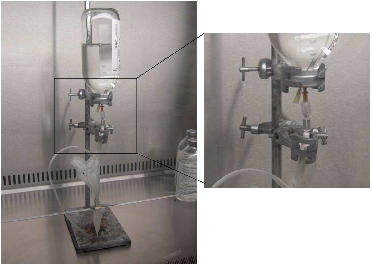
Figure 2.1: Procedure for transferring SAS from manufacturer's bottle to labile plasma pack
