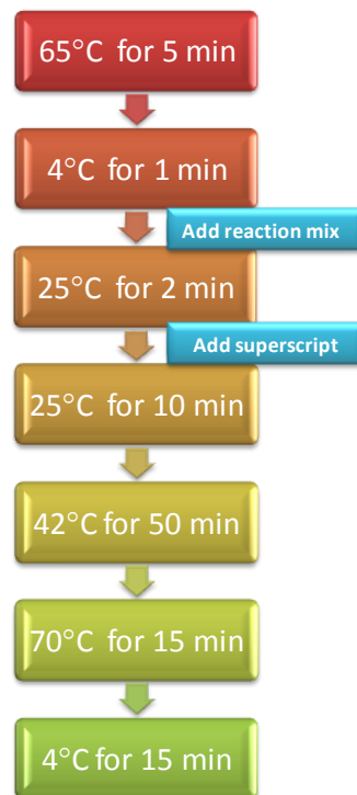
Figure 3: The timing and temperatures used on a thermocycler to convert RNA to cDNA.
