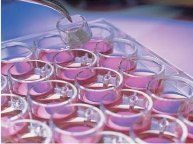
Figure 2.2. Schematic depicting the positioning of a millipore filter insert into a 24 well culture plate.
