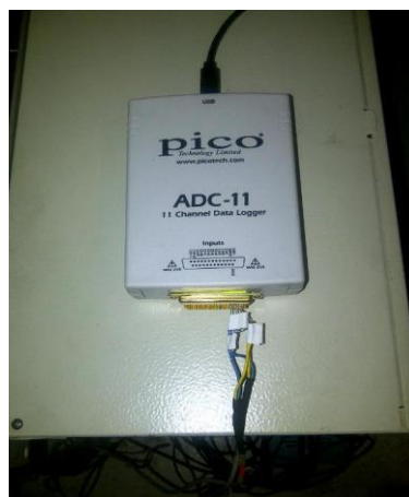
Fig. 5.31 Pico ADC-11 data logger
