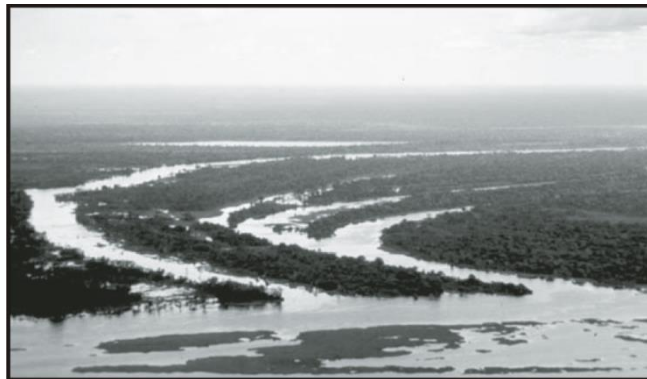
Figure 1.5: Photo illustrating a series of inundated swales from an Amazonian floodplain. The swales can channelise water and potentially lead to chute cutoff (Constantine et al. 2010b).
