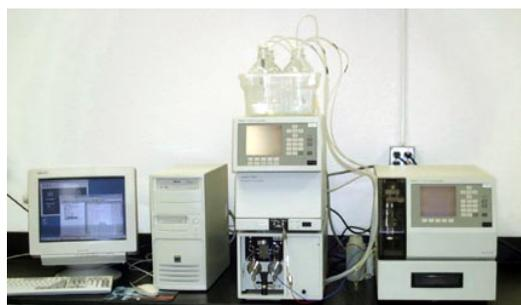
**(Figure 3.3.2a)** HPLC system used in Cardiff University to analyse Actovegin
