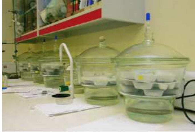
Fig. 3.10 test setup for desiccator tests
