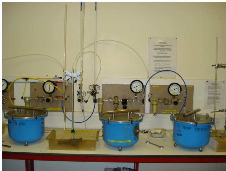
Fig. 3.9 5-bar pressure plate extractor
