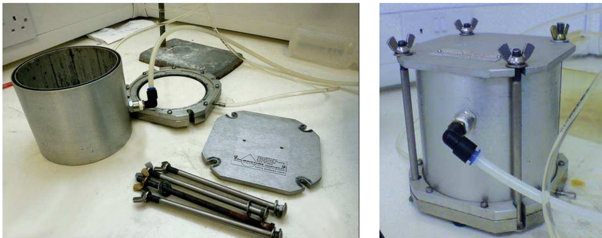
Fig. 3.11 2-bar volumetric pressure plate
