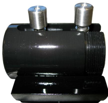
**Figure 2.16.** The sample chamber designed for spectrophotometry study.
