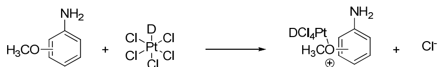
Scheme 3.4. Hypothetical complex formed between platinum (IV) catalyst and oxygen of methoxy group.
