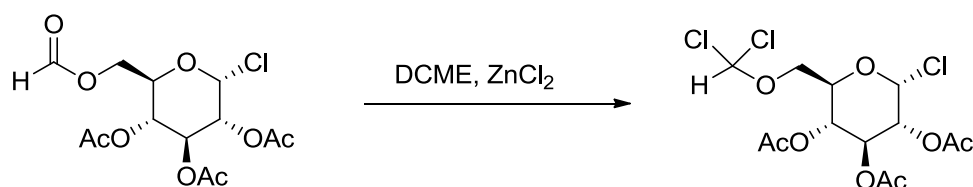
Scheme 2.9 Synthesis of a dichloroalkoxy compound using DCME/ZnCl 2
