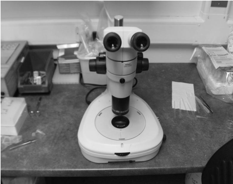
Figure 2.1 Nikon C-DSD230 dissecting microscope used to release and collect eggs.
