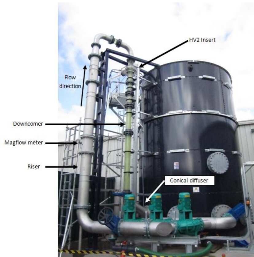
Figure 9.10: - Large scale testing experimental set up.
