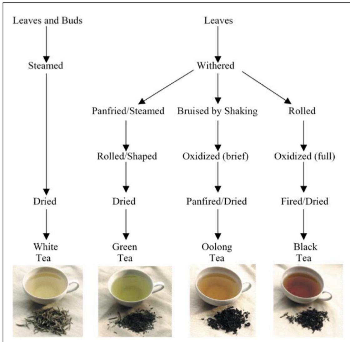
**Figure 1.4.** Processing of different types of common teas (taken from Santana-Rios *et al.*, 2001).
