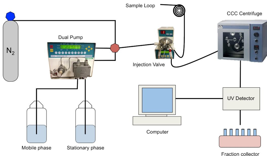
**Figure 4.1.** A schematic diagram of HPCCC equipment and set up.
