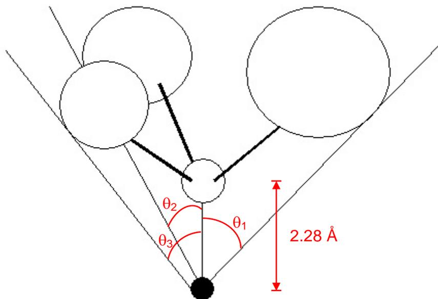
**Figure 1.4** - Tolman Cone Angle,  $\theta$ . The angle measured from the centre of the metal to the edge of the van de waals radii of the outermost atom of the R group <sup>[8]</sup>
