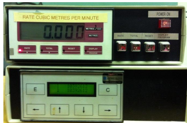
Figure 4-4 Ultrasonic flow metre
