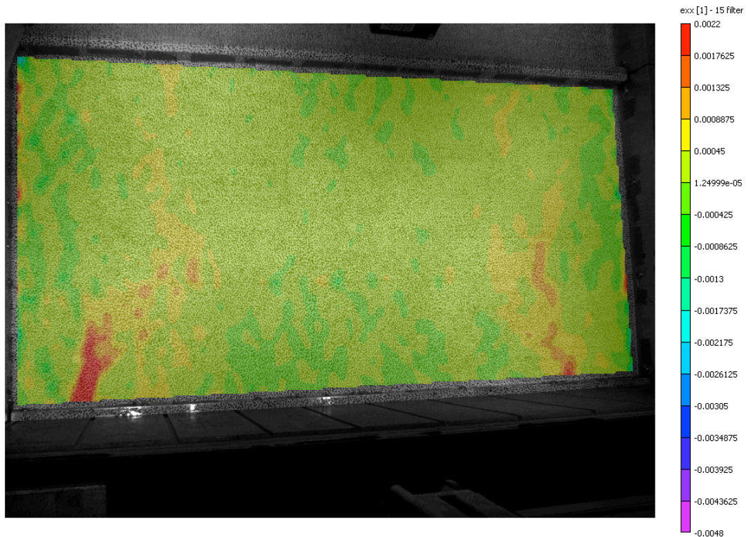
Figure 7.21. Contour plot of strain in the x direction for brick specimen H7 at a water level of 245 mm immediately before failure
