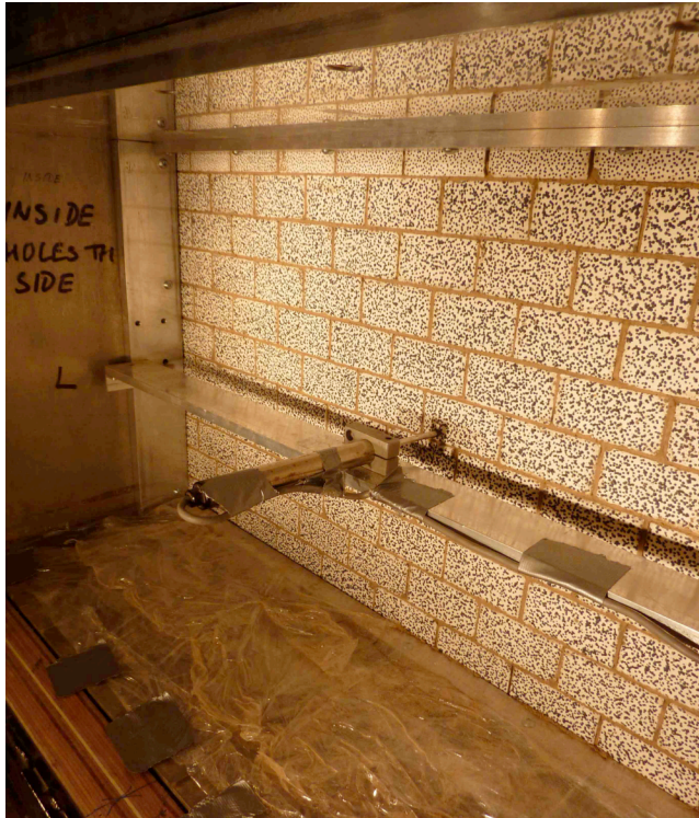
Figure 4.23. View of test jig showing position of LVDT
