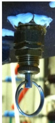
Figure 3.10: Pressure relief valve
