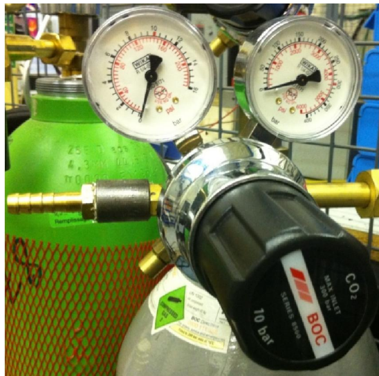
Figure 3.15: CO 2 pressure regulator
