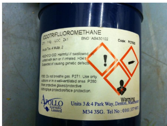
Figure 5.2: CF 3 I description on the bottle
