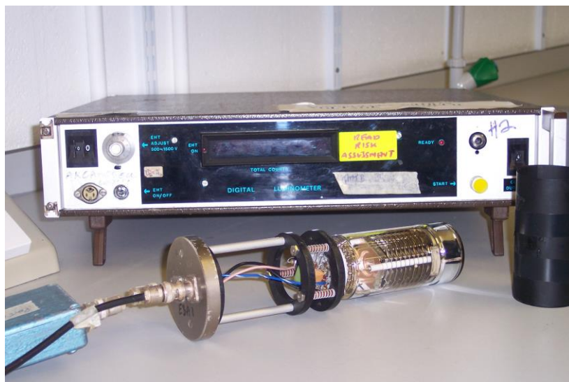
Fig.2.1. The chemiluminometer. The picture shows the photomultiplier tube.
