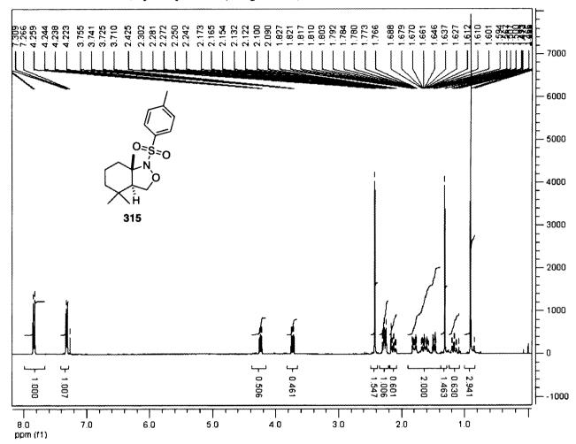
Proton NMR spectrum of bicylic isoxazolidine 315 (400MHz, 300.0°K in CDCl<sub>3</sub>).
