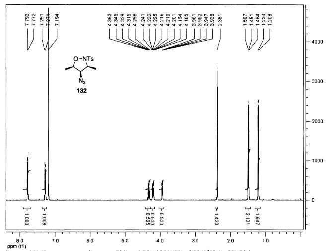
Proton NMR spectrum of isoxazolidine 132 (400MHz, 300.0°K in CDCl<sub>3</sub>).
