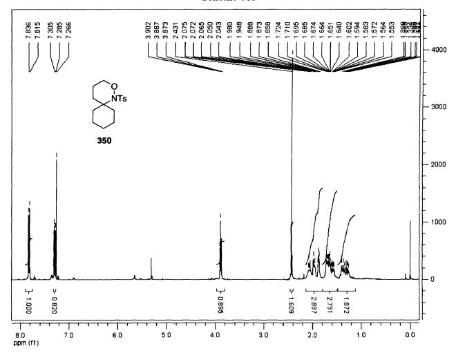
Proton NMR spectrum of crude spiro-cycle 350 (400MHz, 300.0°K in CDCl<sub>3</sub>).
