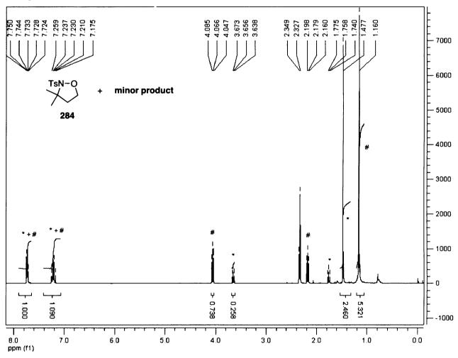
Proton NMR spectrum of crude cyclisation product (Scheme 126), isoxazolidine **284** (#) and an unidentified minor product (\*) (400MHz, 300.0°K in CDCl<sub>3</sub>).
