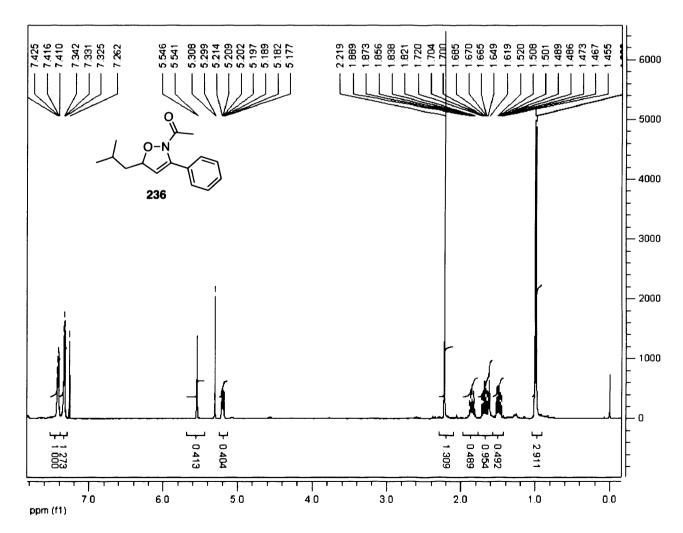
Proton NMR spectrum of dihydroisozazole 236 (400MHz, 300.0°K in CDCl<sub>3</sub>).
