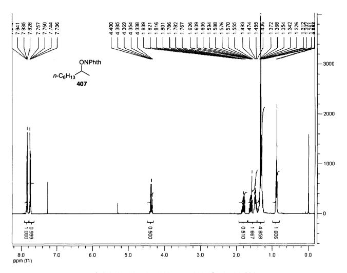
Proton NMR spectrum of phthalimide 407 (400MHz, 300.0°K in CDCl<sub>3</sub>).
