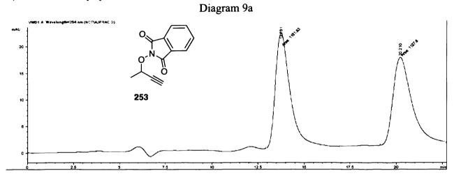
Chiral HPLC analysis of compound 253. Column: OD Chiracel. Flow: 1 ml/min.  $\lambda_{max}$  254 nm. Injection volume: 5  $\mu$ L. Solvent: 10% propan-2-ol, 90% hexane.
