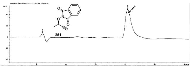
Chiral HPLC analysis of compound 251. Column: OD Chiracel. Flow: 1 ml/min.  $\lambda_{max}$  254 nm. Injection volume: 5  $\mu$ L. Solvent: 10% propan-2-ol, 90% hexane.
