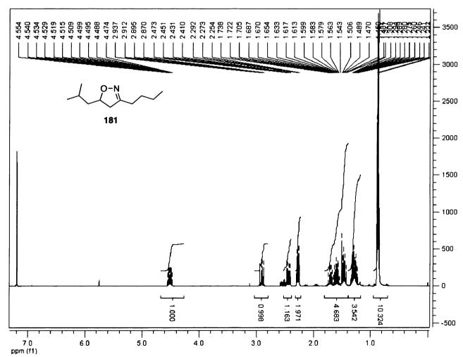
Proton NMR spectrum of crude isoxazoline 181 (400MHz, 300.0°K in CDCl<sub>3</sub>).
