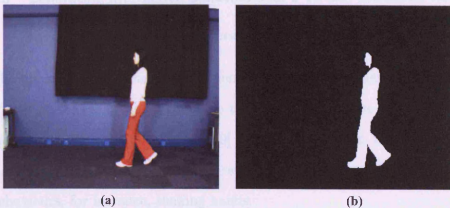
Figure 3.3. (a) Original image of a person, (b) the person in the scene without background.
