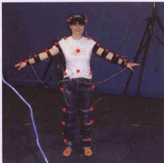
Figure 3.2. Human model with 30 markers (Two markers on the back are not visible).
