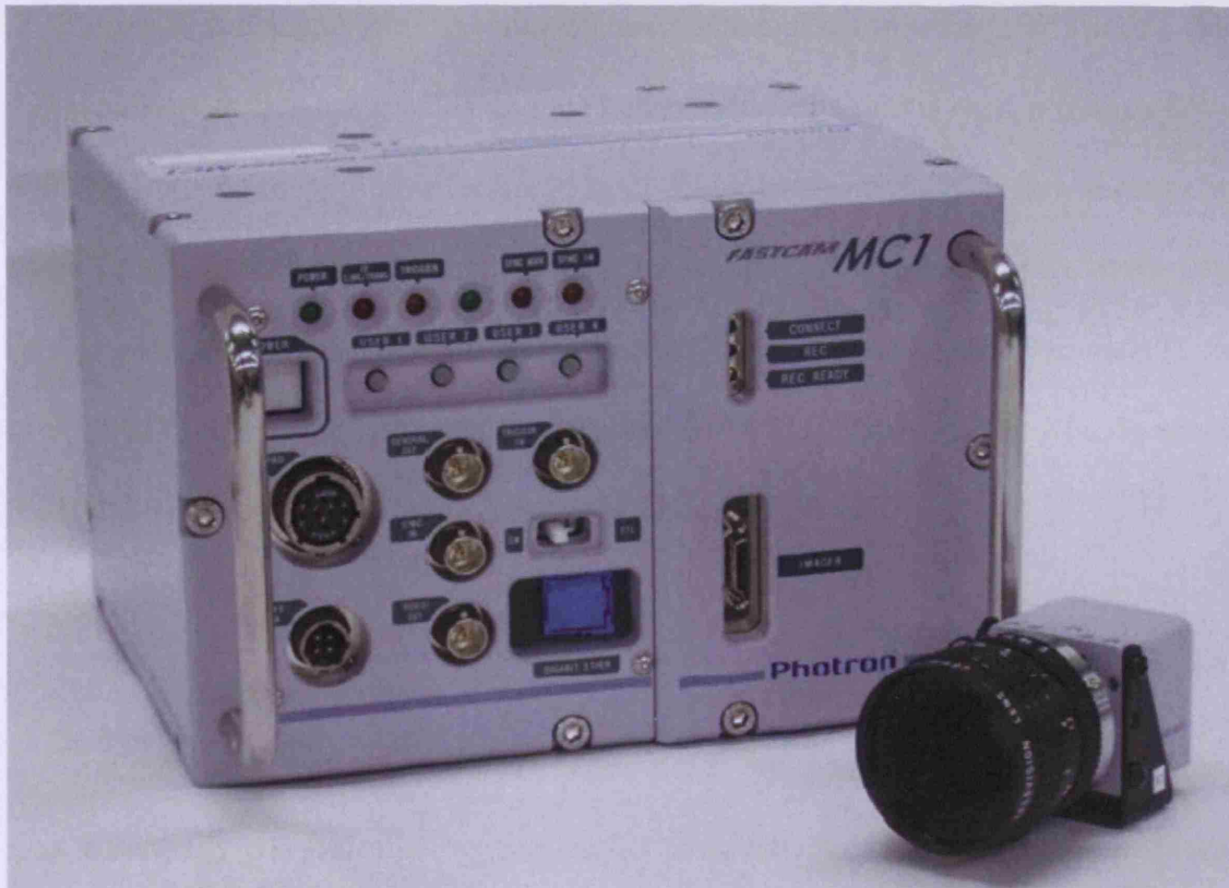
Figure 5.1 The Photron Fastcam MC-1 camera with its processor-controlling unit
