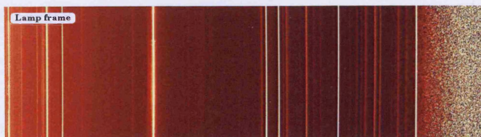
Figure 4.3: An example exposure of an argon calibration lamp used to calibrate the wavelength scale of the science images.
