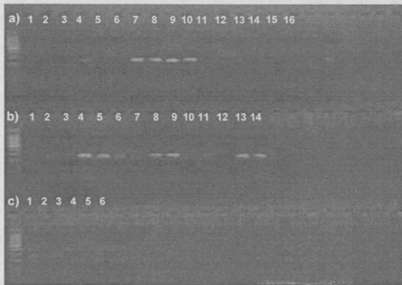
Figure 2.9. Agarose gel electrophoresis picture of DNA amplified from slow worm ( Anguis fragilis ) faecal samples with earthworm-specific 12S primers: 185F and 14233R (Harper et al. 2005). a) Lanes: 1 ( Aphis fabae ); 2 ( Adalia bipunctata ); 3 ( Erigone dentipalpis ); 4 ( Scaeva pyrausti ); 5 ( Forficula sp.); 6 ( Tipulidae sp.); 7 ( Lumbricus terrestris ); 8 ( Aporrectodea caliginosa ); 9 ( Aporrectodea longa ); 10 ( Lumbricus rubellus ); 11 ( Arion intermedius ); 12 ( Deroceras reticulatum ); 13 ( Arion owenii ); 14 ( Limax flavus ); 15 ( Arion hortensis ); 16 ( Metasyrphus luniger ); b) Lanes 1-14: slow worm faecal samples (14 different individuals); c) Lanes 1 and 2: slow worm; lanes 3-6: water (negative control).
