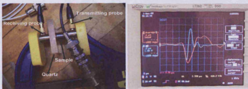
Fig. A1.4: Experimental setup for determining the mechanical properties of cobalt ferrite via the ultrasonic method.
