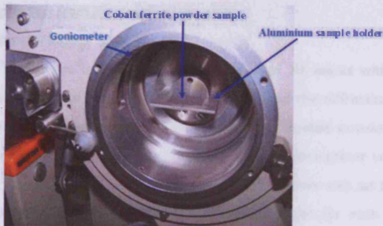
Fig. 5.6: Cobalt ferrite powder sample in the Goniometer for X-ray diffraction
