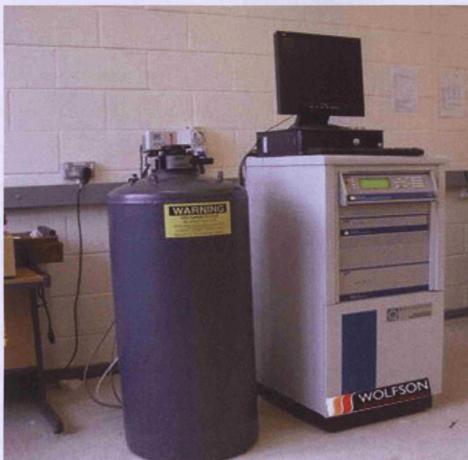
Figure 3-9 The Physical Property Measurement System (PPMS) used to make magnetostriction measurements.
