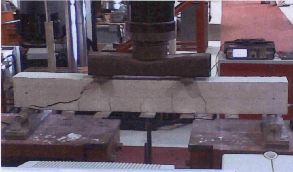
Plat 7.1: Typical shear failure in control beams reinforced only in flexure
