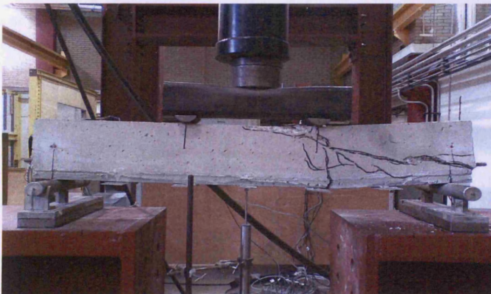
Plate 7.4 Combination shear and flexural failure of retrofitted beam on tension face and without shear reinforce
