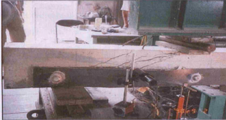
Figure 2.4 Typical failure of RC beam with web-bonded continuous steel plates.
