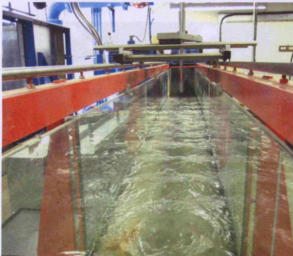
Figure 5.6 View of the small laboratory flume
