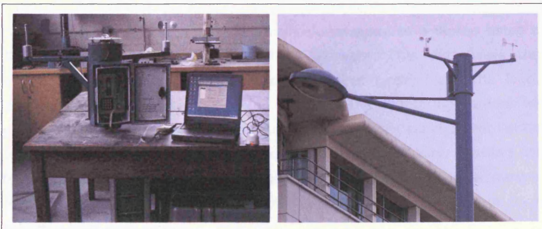
Figure 68: Data monitoring station in lab (left) and in-situ at case study location (right)
