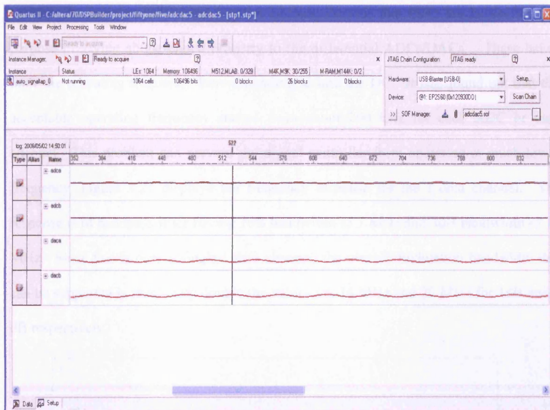
Figure 3.19: STP display waveforms of ADCs input and DAC output
