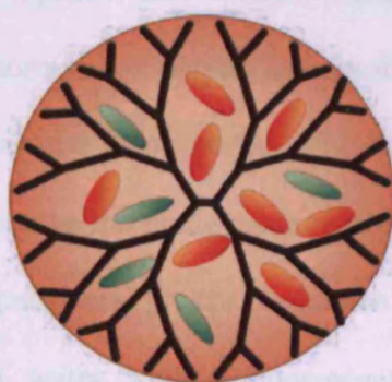
Figure [1.8]: Drawing of a dendrimer carrier encapsulating hydrophobic drug molecules in the dendrimer's voids to increase their aqueous solubility and control their release rate. [15]
