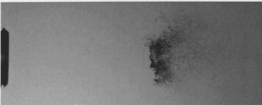
Figure 6.22g: Pulsed Flow Breakup, z=40\text{mm} , Frame 7
