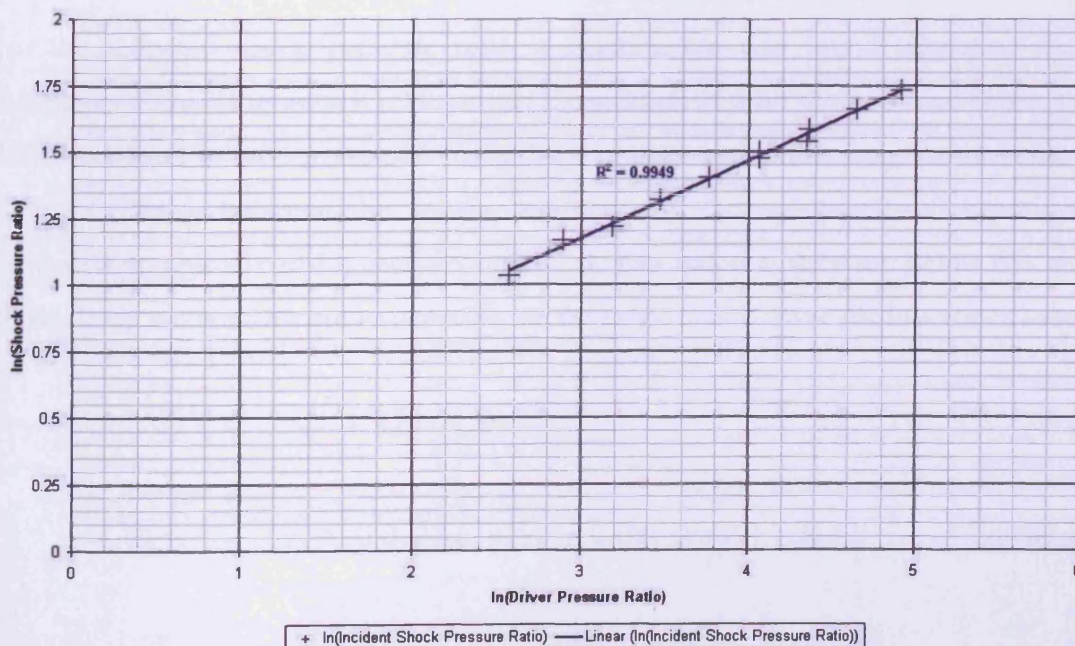
Figure 4.7: log/log Plot of Incident Shock Pressure
