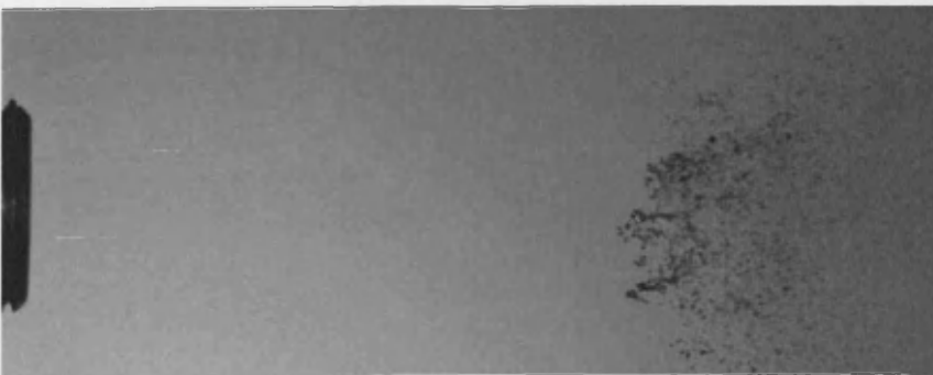
Figure 6.22k: Pulsed Flow Breakup, z=40\text{mm} , Frame 11
