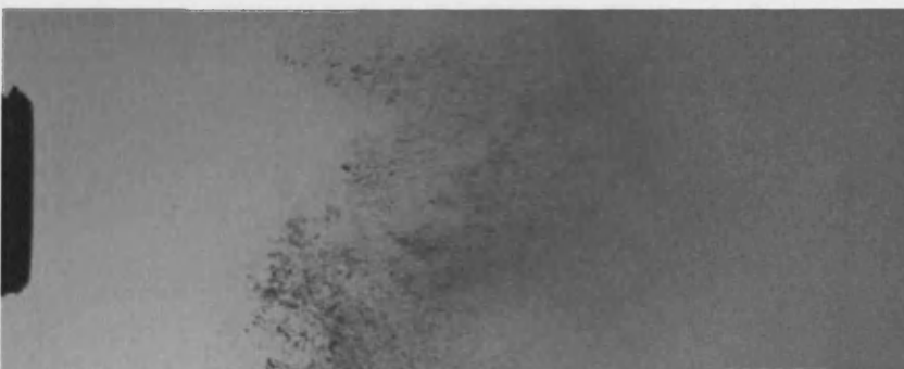
Figure 6.19h: Pulsed Flow Breakup, z=10\text{mm} , Frame 8
