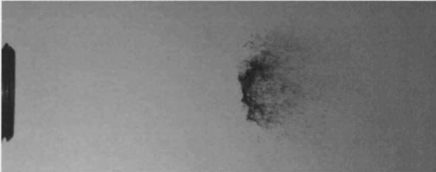
Figure 6.22f: Pulsed Flow Breakup, z=40\text{mm} , Frame 6
