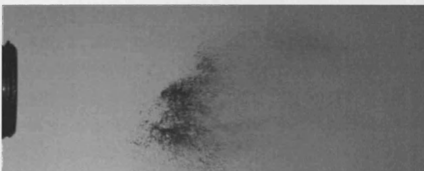
Figure 6.20g: Pulsed Flow Breakup, z=20\text{mm} , Frame 7
