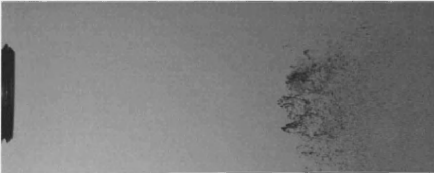
Figure 6.22j: Pulsed Flow Breakup, z=40\text{mm} , Frame 10
