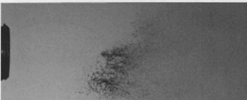
Figure 6.20h: Pulsed Flow Breakup, z=20\text{mm} , Frame 8
