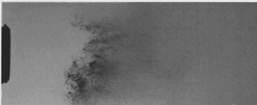
Figure 6.19g: Pulsed Flow Breakup, z=10\text{mm} , Frame 7
