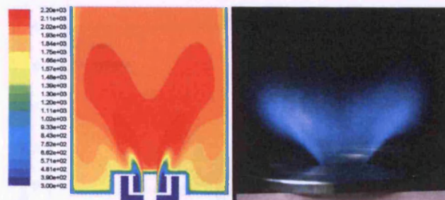
Figure 7. PARTIAL FLASHBACK OF METHANE FLAME IN MODEL AND EXPERIMENTS, \dot{m} = 2.74 g/s, \phi = 0.92
