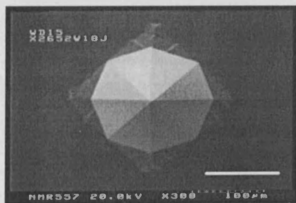
Figure 2. SEM image of an overhead view of a single octagonal wet-etch microneedle. Bar = 100 \mu\text{m} .
