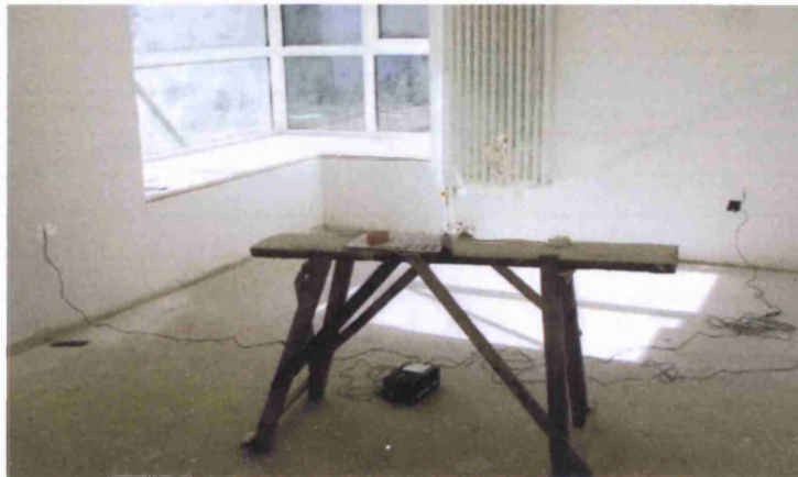
Figure 5. 19: Loggers Placed on a Wood Stand in the Centre of Main Bedroom
