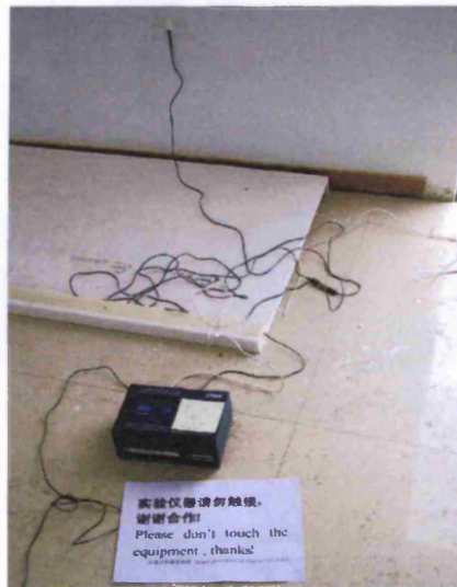
Figure 5. 17: Bead Thermostats were Stuck on External and Internal Walls to Record their Surface Temperature
