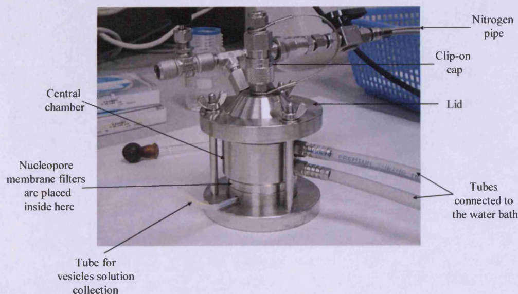
Figure 3.2 Extruder unit used for extrusion of the DPPC vesicles.
