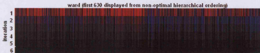
Figure 6.8: Display of mean 'driving' scores through five successive iterations of driving/driven analysis. The tendency of each data point to be of the same sign though smaller magnitude than the same point for the preceding iteration indicates a stable convergence of the algorithm.
