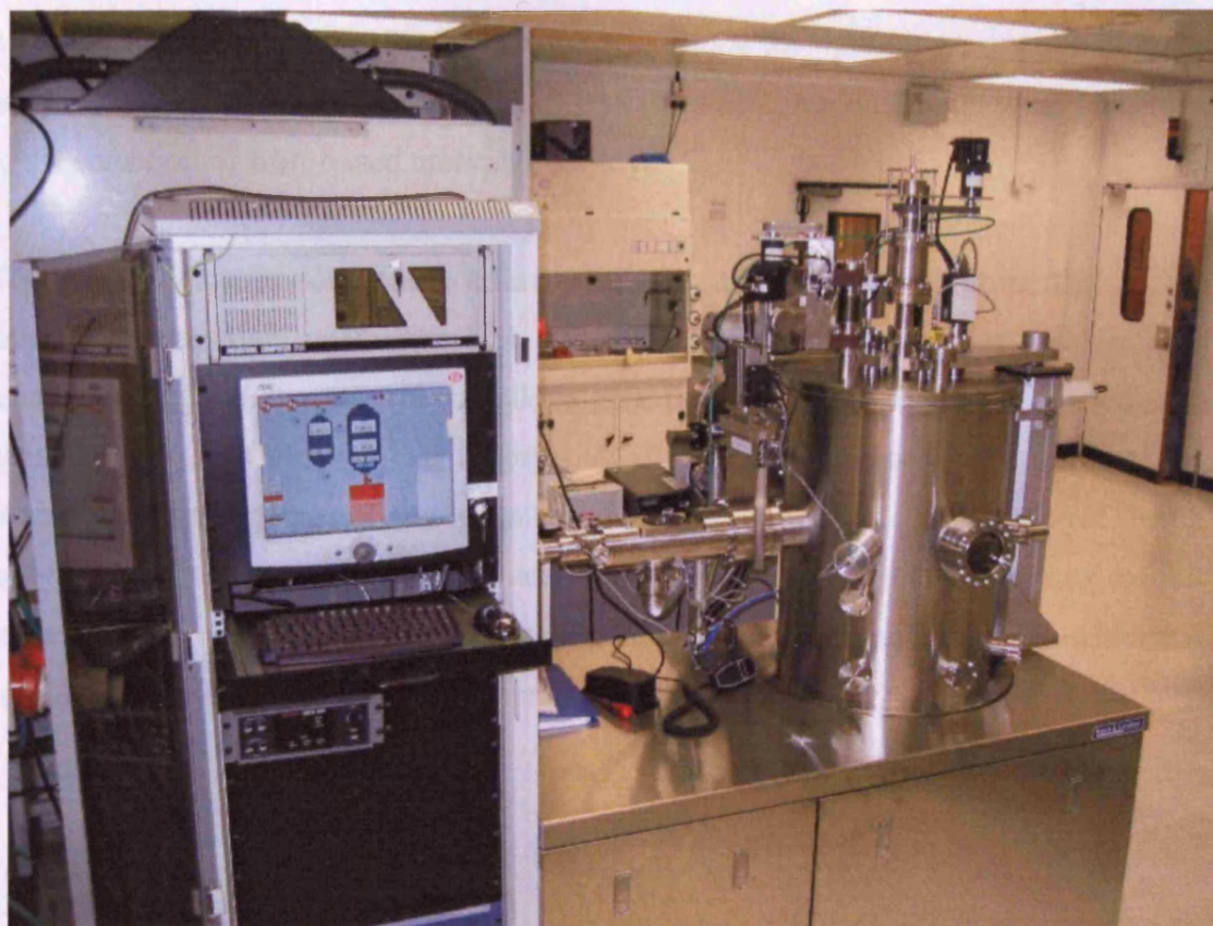
Figure 3.7: The thin film magnetron sputtering system at Cardiff University 17 .
