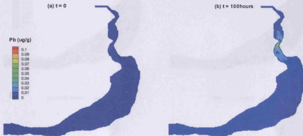
Figure 8-17 Spatial distributions of concentration of trace metal in bed sediment at (a)  $t=0$  and (b)  $t=100$  hours for Case 2
