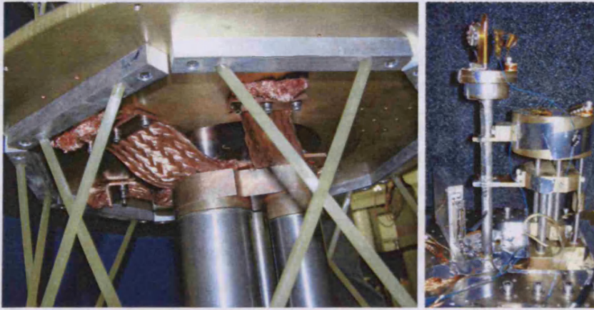
FIGURE 6.4: Clover prototype cryostat's flexible thermal links and base plate support structure, plus the 3-stage sorption refrigerator.
