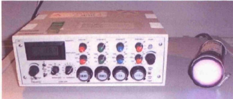
Figure 6.2 LED stimulator used in recording the ERG.
