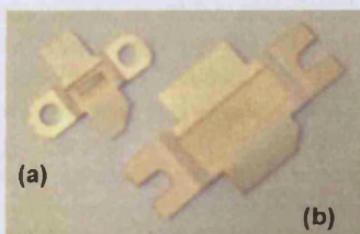
Fig. 9 High Power Laminate Based Packages, (a) 30Watt Package with 30W Device Attached and (b) 100Watt Package.
