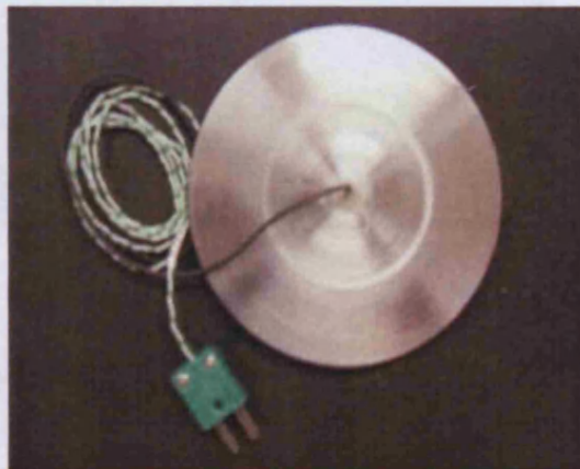
Welded tip teflon thermocouple
