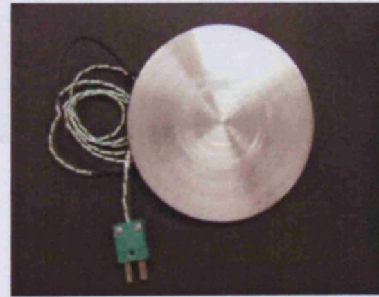
Mineral insulated duplex thermocouple
