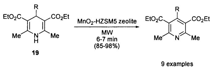
Scheme 36. Oxidative aromatization of 1,4-DHP with \text{MnO}_2 reported by Haravi
