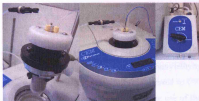
Figure 40. 80 mL flow cell set up (left and centre) and pressure device (right)
