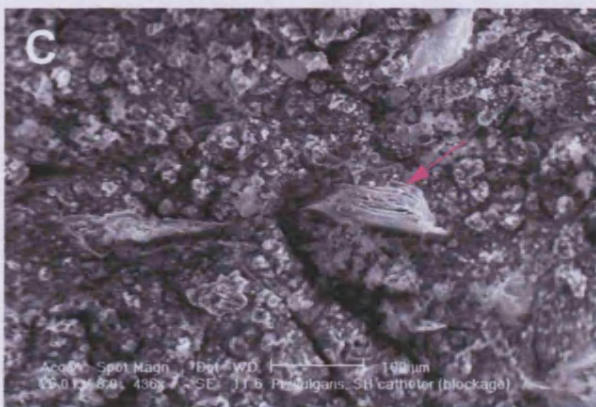
C & D: Encrusted Pr. vulgaris biofilm on a silver-hydrogel catheter. A large struvite crystal is present (indicated by ←, C), surrounded by apatite microcrystals. Few struvite crystals were observed in the biofilm. Pr. vulgaris cells were seen in association with apatite microcrystals at higher magnification (D).
