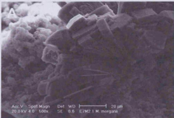
A & B: The crystalline nature of an M. morganii biofilm on an all-silicone catheter (removed from the bladder model after 4 days).
