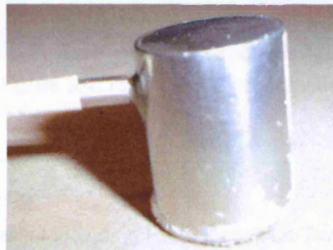
Figure 3.3: Physical Acoustic Corporation type R6D sensor
