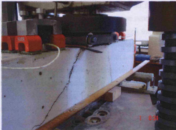
Figure 4.9: Beam failed in shear mode.
