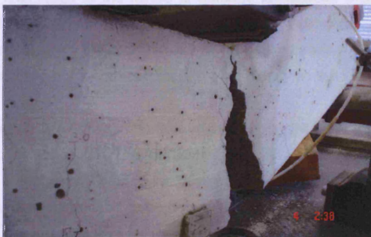
Figure 4.11: Beam failed in flexural mode.
