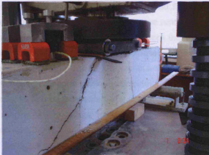
Figure 4.9: Beam failed in shear mode.
