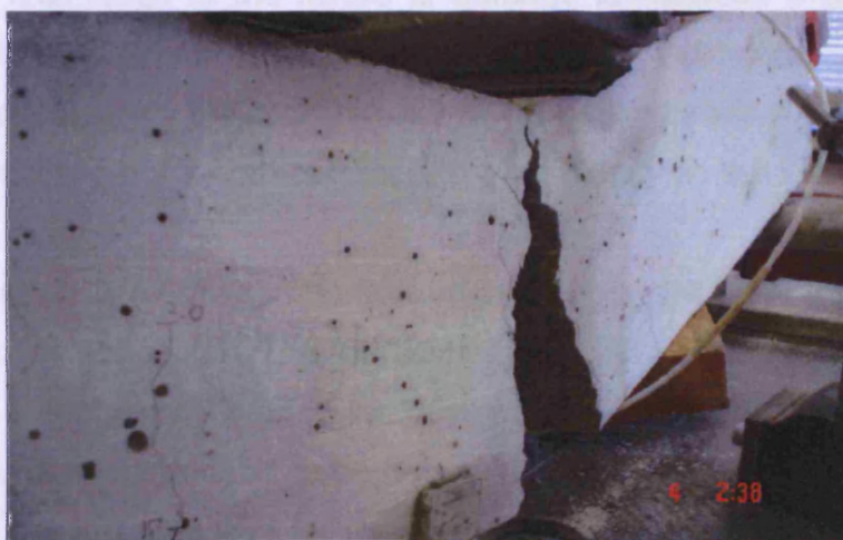
Figure 4.11: Beam failed in flexural mode.
