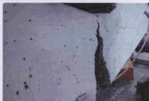
Figures 5a and b above: Beam failed in shear mode and flexural mode.
