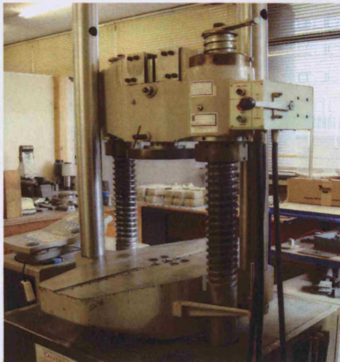
Figure 3.14: Avery-Denison Testing Machine.
