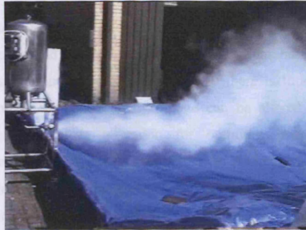
Figure 3.5 Experimental set-up for measuring rainout fraction
