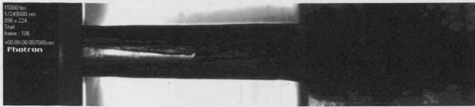
Figure 7.31 Internal and external flow conditions at 131.2°C and 4.7bar
