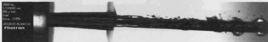
Figure 7.3 Internal and external flow conditions at 121.3°C and 4.9bar
