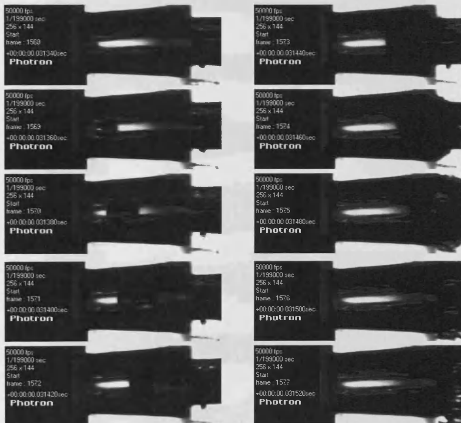
Figure 7.15 Bubble growth inside 2x3.4mm nozzle at 122.3°C and 3.2bar
