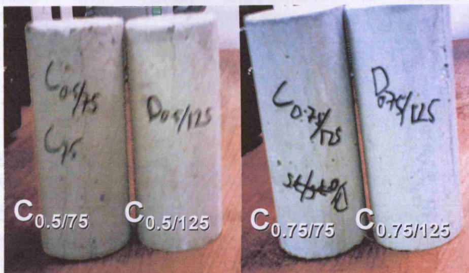
Figure 4.15. Specimen after splitting test for concrete fibre concrete
