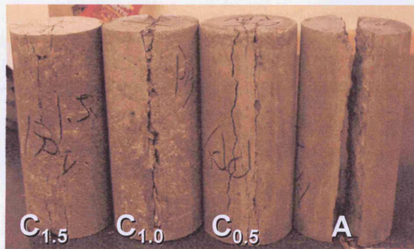
Figure 4.11 Condition of concrete cylinder after splitting test
